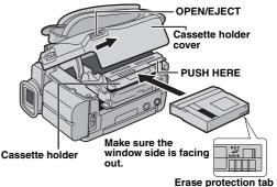
I Slide and hold **OPEN/EJECT** in the direction of the arrow, then pull the cassette holder cover open until it locks. The cassette holder opens automatically.
